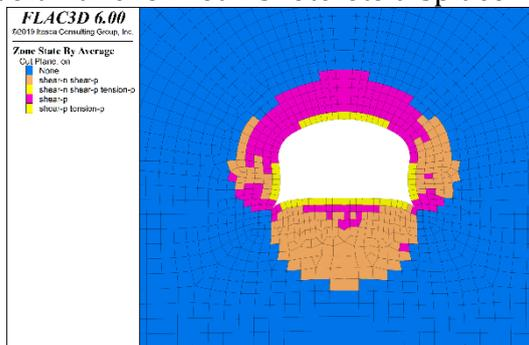
Fig. 4 Distribution of plastic zone of anchor bolt + anchor net + shotcrete
