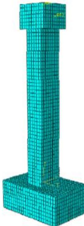
Fig.3 Mesh generation of finite element model
