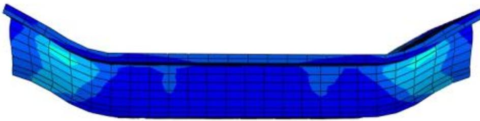
Fig. 7 Mises stress cloud chart of L5 model beam
