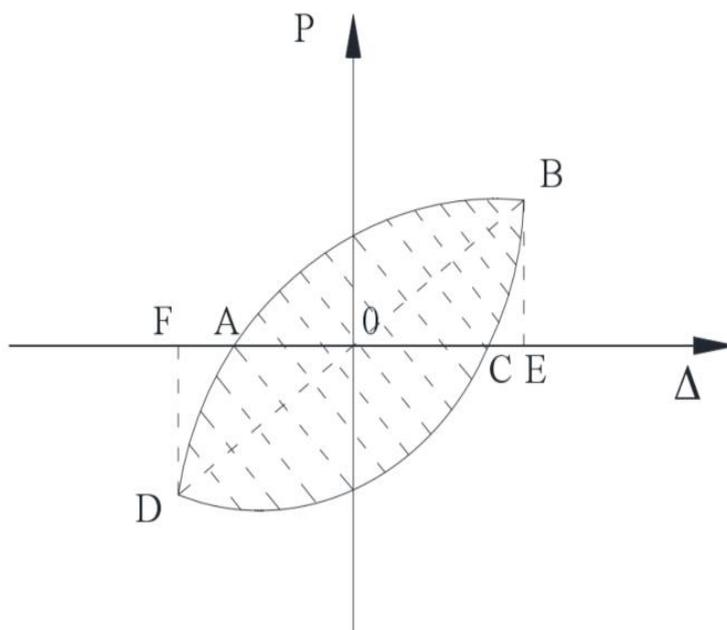
Fig.10 Equivalent viscous damping coefficient calculation sketch map
