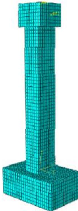
Fig.3 Mesh generation of finite element model
