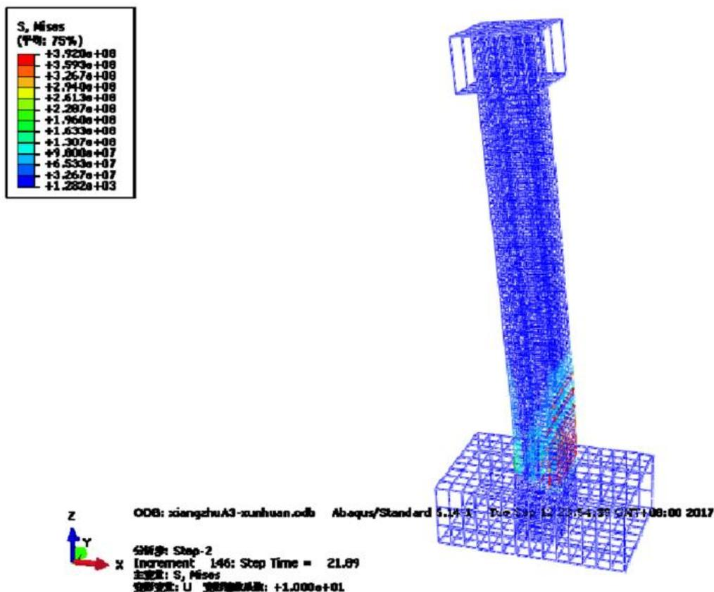
Fig.6 Stress cloud diagram of box column steel bar
