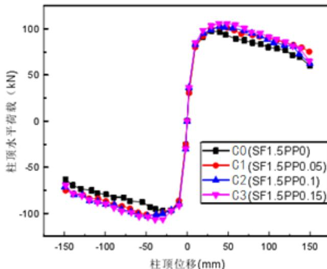
Fig.9 Skeleton curve of fiber concrete box column model
