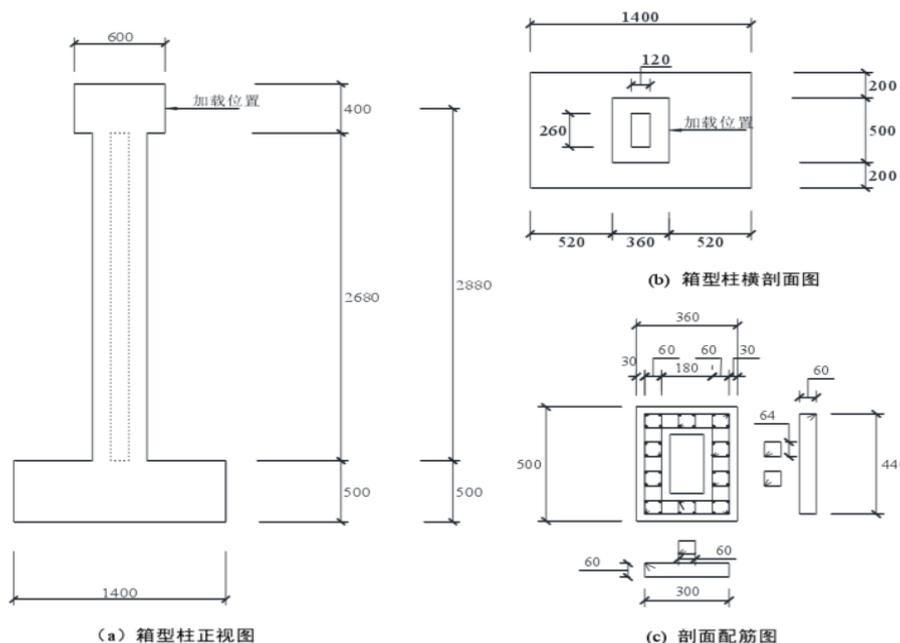
Fig. 1 Size and reinforcement drawing of box column
