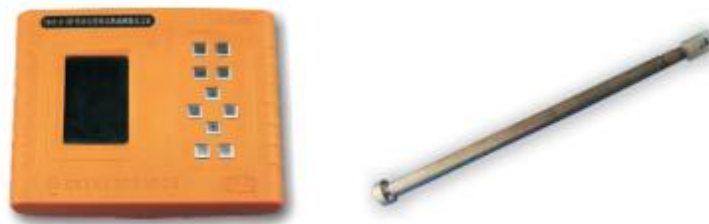
Figure.2 Borehole track measuring instrument of intrinsic safety type used in mine
