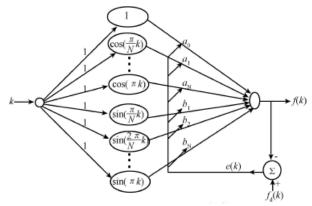
Fig. 1 BP neural network model based on Fourier basis function
