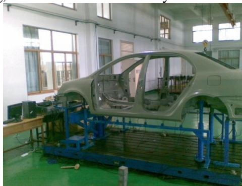
vehicle stiffness test site
