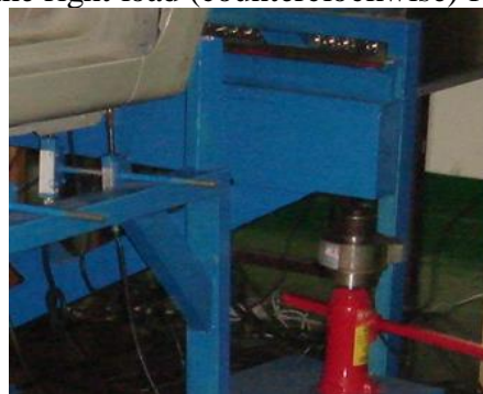
Fig.6 Loading conditions of torsion test
