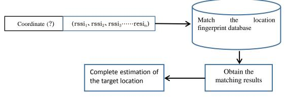
Fig.1 The principle of the fingerprint database positioning stage
