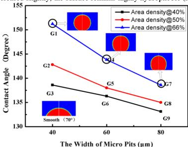
Fig. 4 Surface contact angle vs. micro-texture surface densities.
