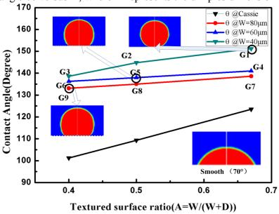
Fig. 3 Contact angle of textured surface under set conditions.
