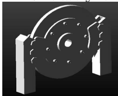
Fig.5 Kinematic model of brake and brake disc
