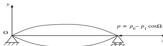
Fig. 1 A model of a simple supported flexible beam at both ends subjected to axial excitation
