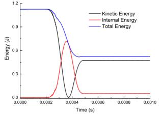
Fig.2 Energy-time history of coal at impact velocity 5m/s
