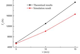
Fig.8 contact force under different impact velocities
