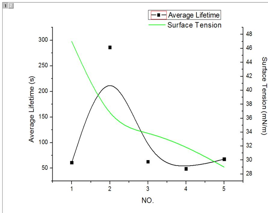
Fig. 8 the changing trend between the surface tension of the solution and the average lifetime of antibubbles
