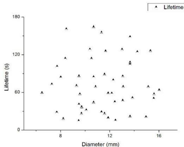
Fig. 1 Relationship between lifetime and diameters of antibubbles in 0.1% volume concentration solution
