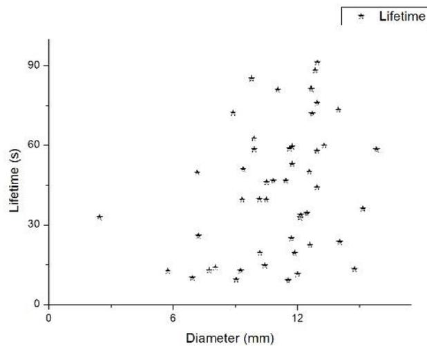
Fig. 4 Relationship between lifetime and diameters of antibubbles in 0.7% volume concentration solution
