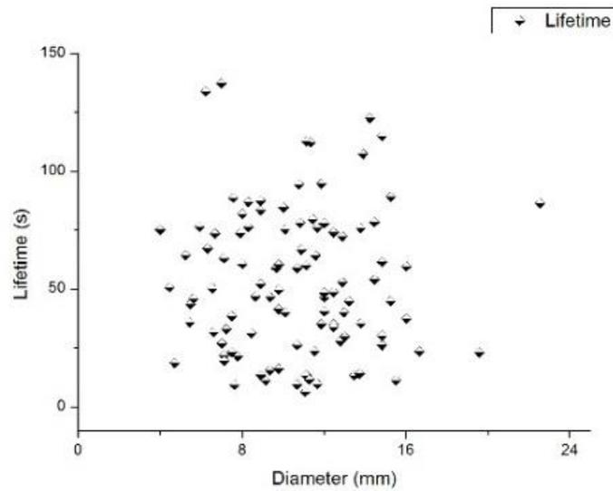
Fig. 3 Relationship between lifetime and diameters of antibubbles in 0.5% volume concentration solution
