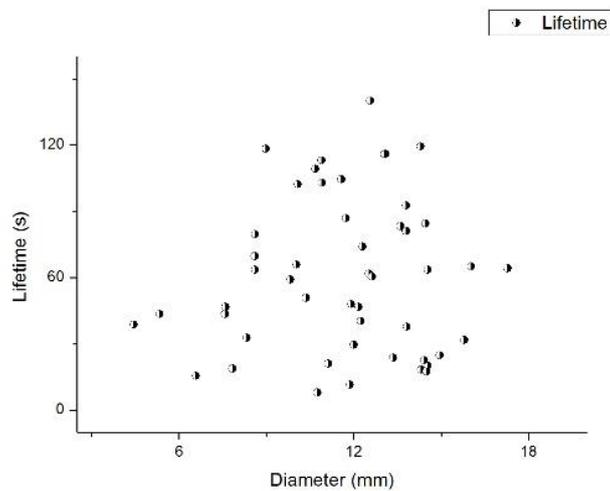
Fig. 5 Relationship between lifetime and diameters of antibubbles in 0.9% volume concentration solution
