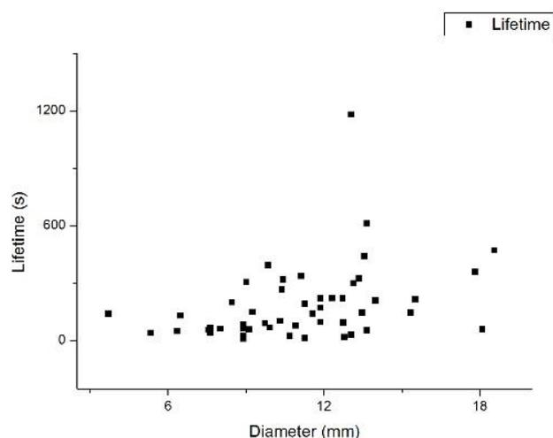
Fig. 2 Relationship between lifetime and diameters of antibubbles in 0.3% volume concentration solution
