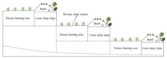
**Figure 1.** An environmentally friendly and structurally stable terrace structure design
