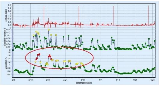
Figure 6. Example diagram of gas gushing warning
